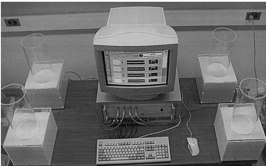
Fig. 2. The 4 detection units in which rats are placed for finch test and the analog input and signal processing module. The computer used in finch detection, display, and analysis is located below the testing table.
