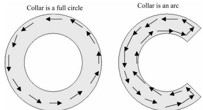
Fig. 4. Representation of current flow occurring with open- and closed-collar configurations.
