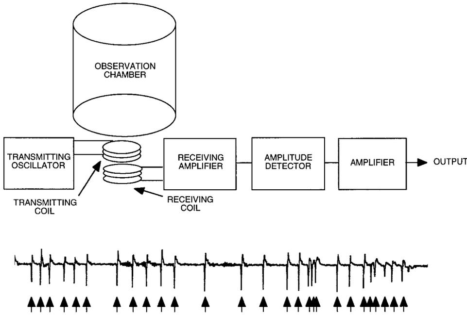
Fig. 1. *Top*: block diagram of the detection unit and its functional elements. *Bottom*: raw signal tracing over 2 min of an animal displaying finch behavior, with arrows added where the processing algorithm detected finches.
